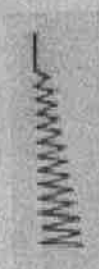
b) needle stitches beginning from the left are directed to the right only
