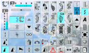
to add a pattern at the beginning of a combination, the cursor must be positioned above the first pattern
