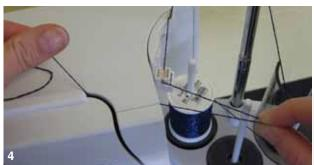
during the initial threading of the sewing computer and when the radial thread release is used it is advisable to pull an extra inch of thread from the spool before the threader button is pushed (Fig. 4)
