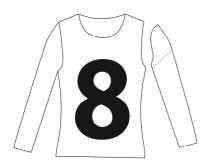
Unpick the sleeve seam. Place the resultant piece on a sheet of paper as a template and trace around it. Now continue working on the paper pattern.
