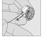
**Insert the bobbin** Insert the bobbin so that the thread runs clockwise.
