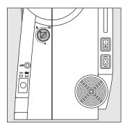
Your sewing computer has been tested and factory set using a double layer of cretonne fabric and Metrosene 100/2 threads (Arova Mettler, Switzerland). Different fabrics, threads and stabilizers can naturally affect the stitch balance so that they are sewn too close together or not close enough. This can be remedied with Balance to suit the fabric and produce perfect results.
