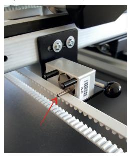
> Place the adjustment weight in the middle of the Frame over both belts.
