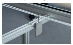
> Tighten **both** setscrews at the X-idler plate **evenly** using the Allen key to tension the X-belt. Make sure that the setscrews are tightenend simultaneously so that the X-belt doesn't run loosely in the idler plate.
