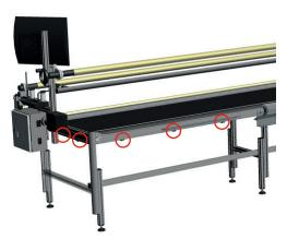
> Lay the cables without any sags and fix them with to every vario-quick holding block with a cable tie.
