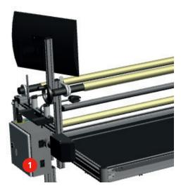
> Turn the red emergency stop knob in arrow direction so that the knob is in the correct position.
