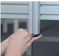
> Insert one hex socket head cap screw through each screwhole at the X-drive and attach the sliding blocks at the hex socket head cap screws loosely by two turns.
