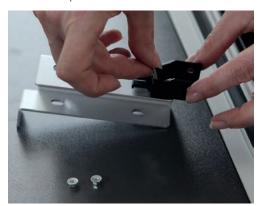
> Loosen and remove the two bottom left screws at the back of carriage.
