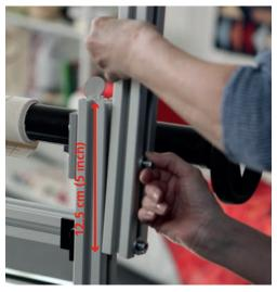
> Also insert two sliding blocks into the previously assembled profile.
