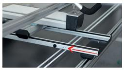
> Attach a 6-kt-hex nuts with flange and serration to each of the button head screws on the backside.
