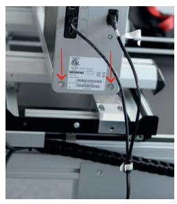
> Insert the previously removed screw into the borehole of the first cable clamp and then place four washers on the screw.
