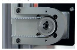
> Place the X-belt along the Frame plate under the machine.
