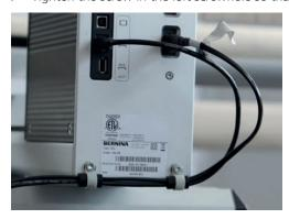
> Wind the spiral cable binding top down around the two cables.
