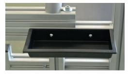
> Insert the hex socket head cap screws with attached washers through both suspensions of the control cabinet and attach the nuts loosely on the other side by two turns.
