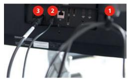
> If necessary, tie all loose cables together with a cable tie and fix them to the Frame.
