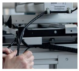
> Insert two cable ties through the **two** openings at the holder of the carriage and around the cables, tie them and cut the ends.
