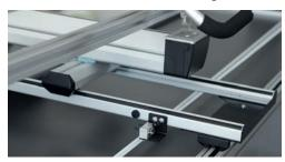
> Position the X-support so that the black pins are flush with the belt at the front.
