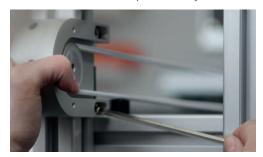
> Place the protective cap under the X-belt to adjust the height of the belt.
