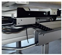
> Fix the energy chain at the security holder with a cable tie as shown in the illustration.
