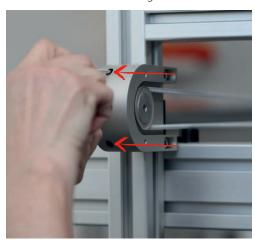
> Tension the X-belt so that there will be an air gap (min. 0.1 - max. 1.0 mm / 0.004 - 0.04 inch) on the adjustment weight between the two belts.
