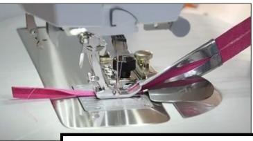
Make adjustments shown as needed the first time you use the binder. Occasional adjustments may be needed as the moving parts of the binder may shift slightly with use.
