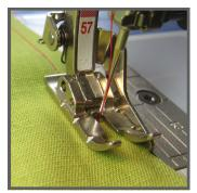
work Foot #37/37D because of a spring-loaded seam guide along the right edges of the 57 feet. The guide ensures perfect 1/4" seams and the spring-action allows the guide to move easily over bulky seams. Especially helpful for beginners, this guide also offers extra insurance to experienced piecers.
