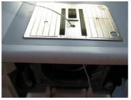
Thread narrow cord through bobbin area and up through hole in front of needle opening (works with models that have the type of stitch plate shown)
