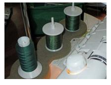
thread in the needle. (See settings on page 1.) Place spool caps over the sewing thread spools.  Stitch a test swatch using the two napkin fabrics. The rolled edge looks a bit different on the top and bottom, so use the swatch to select which fabric will be on
