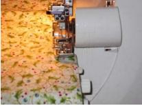
Tip: Prevent "dog ears" (pointy corners) by making sure fabric feeds through straight at corners and doesn't slide to one side.
