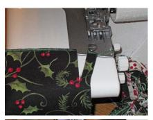
Raise the presser foot and position the fabric as if the fabric had been cut with the serger knife, with the bulky edge next to the needles.
