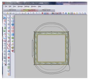
• Select the Hoop Layout Tab and add hoops to the left and right to cover the entire border design. Select Calculate Hoopings, which should result in three hoopings. The BERNINA Embroidery Software 6 will split the border into separate sections to fit the selected hoop and insert reference marks as guides for aligning the designs.
