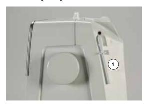
The vertical spool pin is on the side behind the handwheel. It is an essential aid for sewing with more than one thread, e.g. double needle work and can also be used for winding the bobbin while sewing.
