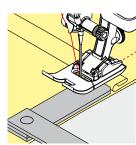
To solve this problem, place one, two or three compensating plates as required behind the needle under the presser foot to level it.
