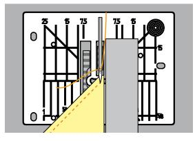
When sewing corners only a small section of the fabric is actually on the feed dog. Therefore it cannot grip the fabric well.
