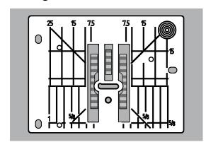
Due to the width of the stitch plate hole the outer feed dog rows are relatively far apart.
