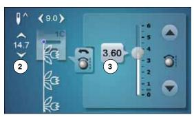
With other stitch patterns, including alphabets, the overall length of a stitch pattern  ${\bf 2}$  is displayed. The actual stitch length  ${\bf 3}$  is visible when the stitch length Display is opened.
