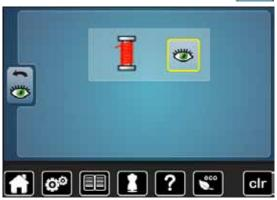
The following monitoring function can be activated or deactivated: Upper thread indicator
