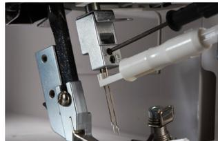
To handle the needle conveniently use the Needle Threader / -Inserter which is provided in the Accessories Storage.
