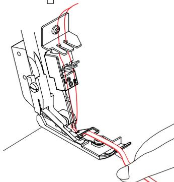
The standard presser foot is equipped with a tape guide. A tape can be sewn into the shoulder or side seams of garments made from knitted or stretch fabric so that losing shape can be avoided.
