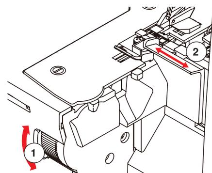
The knife position and as a consequence thereof the resulting cutting width can be adjusted between 3 - 9 mm by turning the cutting width dial at the front of the sewing table. The set cutting width is shown on the cutting width indicator (2). The scale indicates the distance of the knife to the left needle (5 - 9 mm). The distance to the right needle is 2 mm shorter.
