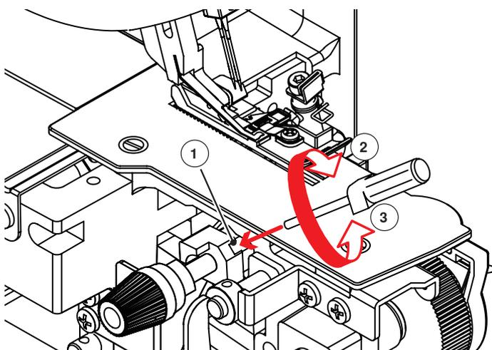
A wide range of fabric can be processed on this machine. When sewing extra heavy weight fabrics or multiple layers of fabric, it is recommended to secure the knife suspension mechanism as following:
