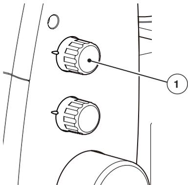
Turn the Stitch Length dial until the desired length is obtained. The higher the number, the longer the stitch. The stitch length is infinitely variable and can be adjusted from 0.8 - 4.0 mm, even while sewing. Adjustments can be made while sewing.
