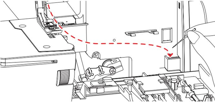
By threading the left needle a seam width of 5-9 mm will be produced. By threading the right needle a seam width of 3-7 mm is generated.
