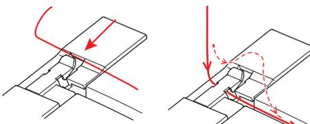
The thread pretensions are on the top of the machine. They are color-coded and simple to thread. Hold the thread with both hands and slip into the appropriate guide from the right side. Then gently pull towards the front, making sure the thread is firmly locked in the pretension hooks.
