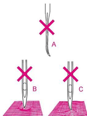
Needles must be in perfect condition to achieve best sewing results. Please check the needles before each sewing project. Defective needles may not only damage the sewing project, but can also damage the overlocker.
