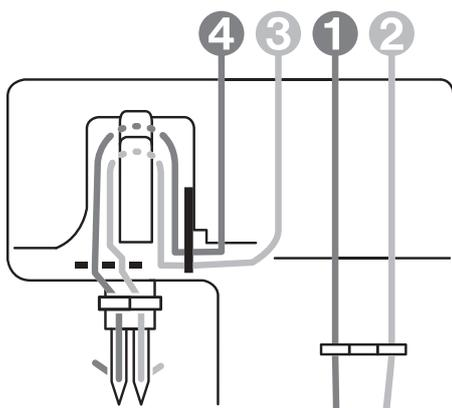
Thread the machine carefully and in the sequence as indicated on the following pages. To achieve a good sewing result, it is important that you follow the sequence as described and as indicated on the Threading Chart (color dots 1 – 4) in the machine.
