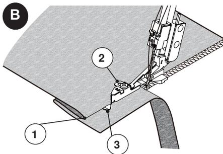
**B** Place the fabric under the presser foot with the 'wrong' side up. Feed the folded edge through the guide (3) in front of the foot and lower the presser foot. Sew the first stitch (or a number of stitches) on a spare part of the original fabric and adjust the guide so that the needle only marginally pierces the folded edge. Adjust the guide by means of the small screw (2) on the top of the foot. When the guide is correctly set, sew the hem. The outside edge will be cut away.
