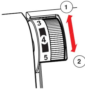
The thread tension can be altered for every thread via the thread tension adjustment.
