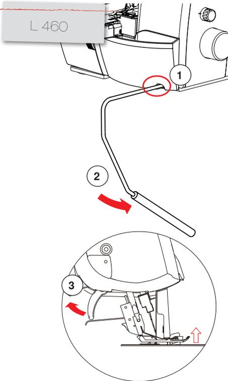
The Free Hand System lever allows raising the presser foot without using the hands.
