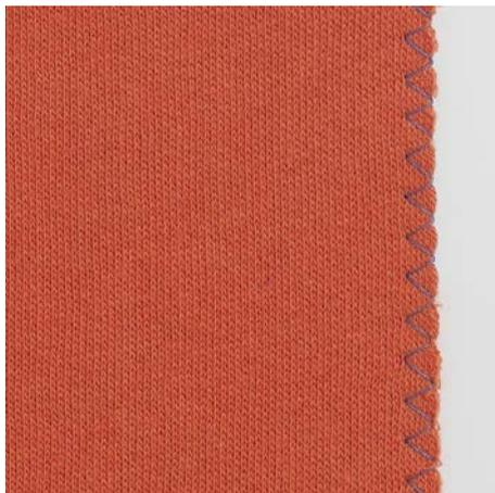
Zigzag No. 2 is suitable for all fabrics. It can be used for elastic seams as well as for decorative work. Use darning thread for fine materials.
