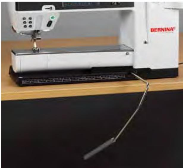
The FHS is used to raise and lower the Presser Foot.
