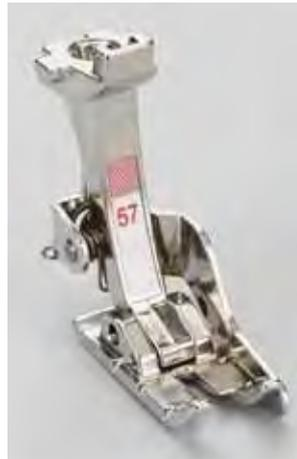
Accuracy is essential when sewing patches together. The side edges of the Patchwork foot are exactly 1/4" (6mm) from the center needle position. The center indents on either side of the foot indicate the needle insertion point and the two additional indents are 1/4" (6mm) in front of and behind the needle. When sewing at a foot's width, the seam allowances will always be the exact width and it is easy to turn the work while maintaining the same width.
