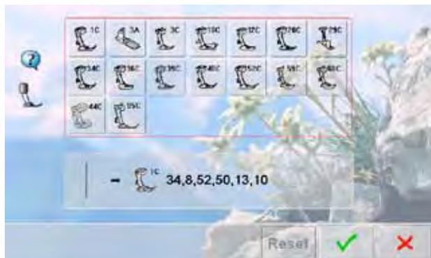
▶ in the opened presser foot category, select the icon that shows the attached presser foot, and confirm ✓. As an alternative, attach one of the options shown in the lower portion of the screen, select the respective presser foot icon and confirm ✓
