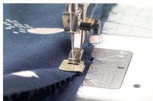
The slot in the foot is used to gather a ruffle and stitch it to a flat piece of fabric all in one operation. The fabric to be gathered is fed under the foot and the flat piece of fabric is fed into the slot, keeping it from touching the feed dog.
