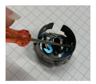
Check the side to make sure the prongs are in the correct place.
