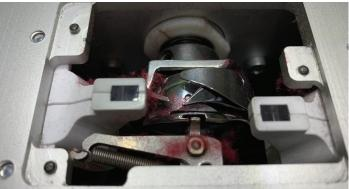
Brush the lint out of the area behind the front door. A large brush may make this easier and faster than the small one used in the bobbin area.
