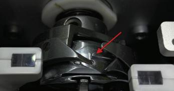
Place one drop of oil so that it will run down the top and sides of the ridge.
