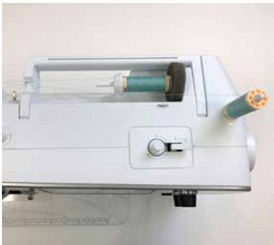
LOADING TWO SPOOLS OF THREAD ON UPPER PART OF MACHINE
