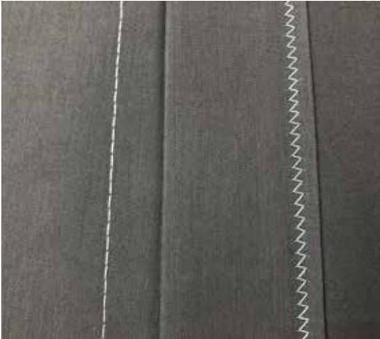
COMPARING WRONG SIDES OF STRAIGHT STITCH SINGLE NEEDLE AND TWIN NEEDLE
