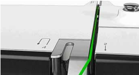
THREADS ON EITHER SIDE OF TENSION DISK
