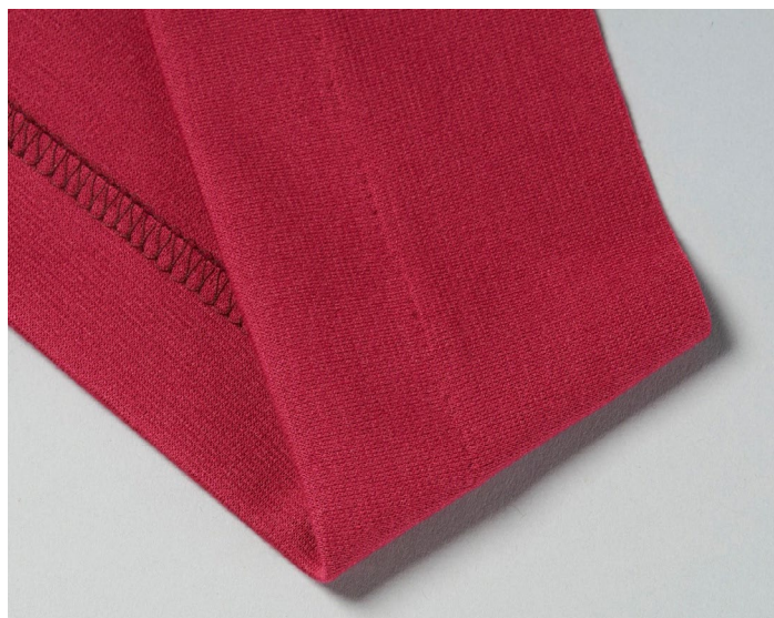
Use the 3-thread overlock with Blindstitch Presser Foot to create a blindhem using an overlocker
