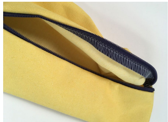
Install a zipper with an overlocker for a clean finished edge
