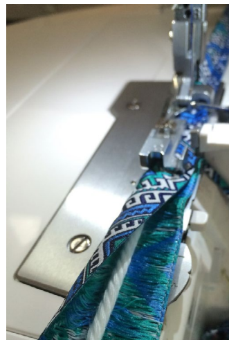
Use a 3-thread overlock and the Multi-purpose Foot to create piping from ribbon
