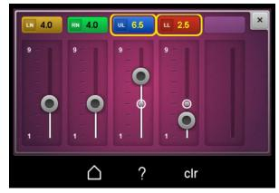
For more control of the tension settings, use the fine adjustment buttons located the front of the machine (manual button). Press the top button for a higher tension and the bottom button for a lower tension. This will move the tension in decimals of 1/10. Thread tension can be adjusted between 1-9 for each stitch. Changes made using the manual buttons will be reflected on the screen.
