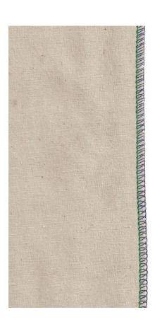
For this exercise, you will thread the overlocker for a 3-Thread Narrow Overlock stitch using the Right Needle and thread colors to match the color-coded threading path on the overlocker. Adjust all thread tension settings for a balanced stitch as indicated below.
