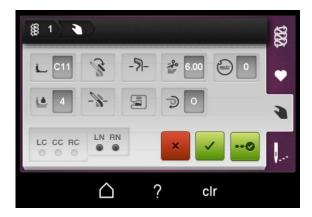
The Wizard can be launched at any time from this screen by selecting the icon. This will walk you step-by-step through all the changes that need to be made for the stitch selected.
