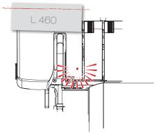
When the Safety LED is activated, the machine will not run.
