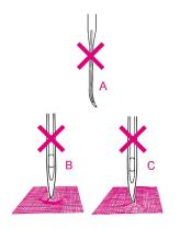
Needles must be in perfect condition to achieve best sewing results. Please check the needles before each sewing project. Defective needles may not only damage the sewing project, but can also damage the overlocker.
