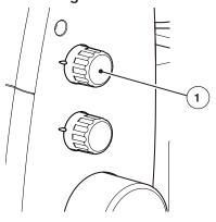
Turn the Stitch Length dial until the desired length is obtained. The higher the number, the longer the stitch. The stitch lenght is infinitely variable and can be adjusted from 0.8 - 4.0 mm, even while sewing. Adjustments can be made while sewing.
