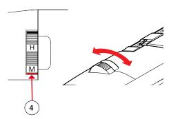
For easy operation adjust the presser foot pressure only with lowered pressure foot.
