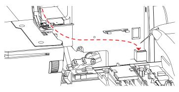
By threading the left needle a seam width of 5-9 mm will be produced. By threading the right needle a seam width of 3-7 mm is generated.
