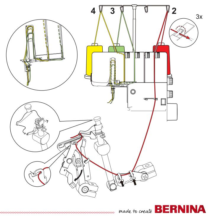
3-thread overlock (LN) (Left needle)
