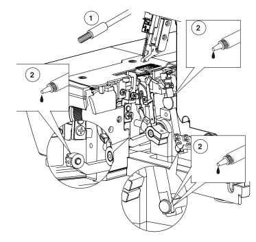
To keep the machine running smoothly, keep it clean at all times and lubricate regularly.
