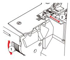
The knife position and as a consequence thereof the resulting cutting width can be adjusted between 3 - 9 mm by turning the cutting width dial at the front of the sewing table. The set cutting width is shown on the cutting width indicator (2). The scale indicates the distance of the knife to the left needle (5 - 9 mm). The distance to the right needle is 2 mm shorter.
