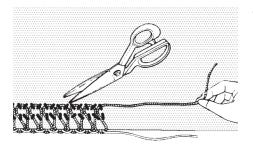
To remove stitches already sewn, snip off the needle thread(s) at intervals and pull out looper thread(s).
