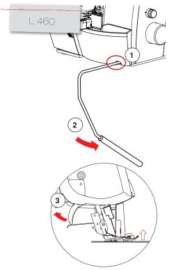
The Free Hand System lever allows raising the presser foot without using the hands.
