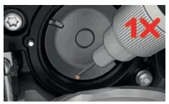
> Add one drop of oil into each of the two oil depots so that the felts are damp, and make sure that the red-marked surface of the hook sleeve remains free of oil.
