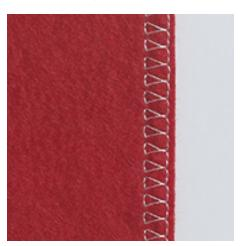
A double overlock seam is suitable for looser knit fabric and for cross seams in woven fabric. When working with jersey, a jersey needle should be used to prevent damaging the knit fabric. When sewing stretch materials, use a stretch needle.
