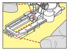
> Pull the cord to the front on the left side under the Buttonhole Foot with Slide.
