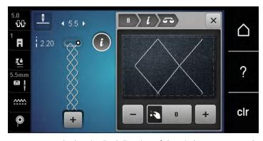
> To correct the longitudinal direction of the stitch pattern, turn the «Lower Multi-function knob» until the preview of the stitch pattern matches the stitch pattern sewn on the fabric.
