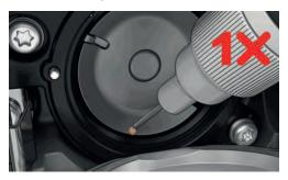
> Add one drop of oil into each of the two oil depots so that the felts are damp, and make sure that the red-marked surface of the hook sleeve remains free of oil.
