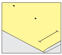
> For keyhole and round buttonholes mark the length of the bead with chalk or a water-soluble pen on the fabric. For any subsequent buttonholes mark the starting point. The length of the keyhole is sewn additionally.
