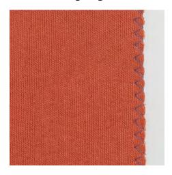
Zigzag No. 2 is suitable for all fabrics. It can be used for elastic seams as well as for decorative work. Use darning thread for fine materials. When sewing satin stitch, it is recommended to set a short, dense zigzag at a stitch length of 0.3 - 0.7 mm. The satin stitch can be used for appliqué and for embroidering.
