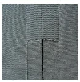
The Triple straight stitch is especially suitable for durable seams and for firm, densely woven fabrics such as denim and corduroy. For firm or densely woven materials it is recommended to fit the Jeans Foot #8. This will help to sew denim or canvas. For decorative topstitching, the stitch length can be elongated.
