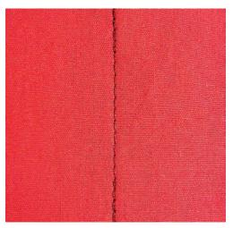
Due to a determined number of 6 stitches sewn forwards and 6 stitches sewn in reverse, the securing is regular.
