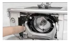
> Fold down the fastening bracket along with the black hook race cover.
