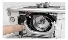
> Fold down the fastening bracket along with the black hook race cover.
