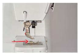
> Lower the shaft via the lever.
