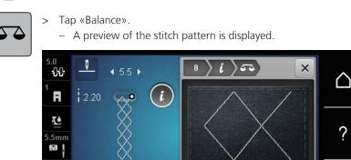
> To correct the longitudinal direction of the stitch pattern, turn the «Lower Multi-function knob» until the preview of the stitch pattern matches the stitch pattern sewn on the fabric.
