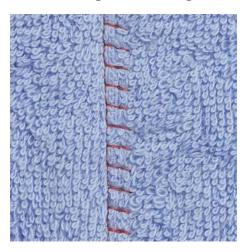
The flat joining seam is especially suitable for long-pile or thick materials such as terrycloth, felt or leather.
