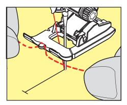
> Pull both cords ends under the Buttonhole Foot to the back and place each a cord into a groove of the sole.
