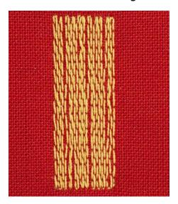
The Simple Darning Program No. 22 is particularly suitable for quick darning of worn areas or tears. It is recommended to use fine material as a backing for the worn and damaged areas or to stick an adhesive interlining. The Simple Darning Program No. 22 replaces the longitudinal threads in all fabrics. If the darning area becomes distorted, correct with the balance.
