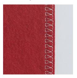
A double overlock seam is suitable for loose knits and cross seams in knits. When working with jersey, a jersey needle should be used to prevent damaging the knit fabric. When sewing stretch materials, use a stretch needle.
