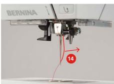
> Pull the thread below the presser foot and through to the thread cutter (15), and cut it.
