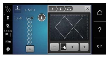
> To correct the longitudinal direction of the stitch pattern, turn the «Lower Multi-function Knob» until the preview of the stitch pattern matches the stitch pattern sewn on the fabric.
