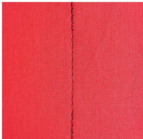
Due to a determined number of 5 stitches sewn forward and 5 stitches sewn backward, the securing is regular.
