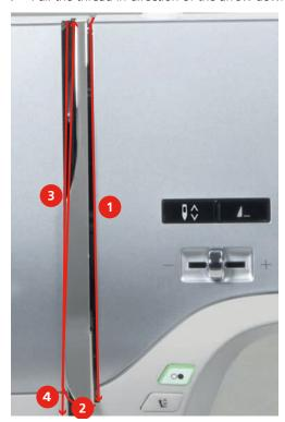
> Guide the thread through the guides above the presser foot.
