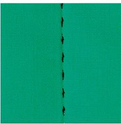
Handlook quilt stitches are suitable for all fabrics and sewing projects which should look «hand sewn». It is recommended to use a monofilament thread as upper thread and an embroidery thread as bobbin thread. The sewing speed should be moderate to prevent the monofilament from breaking. If required, the upper thread tension and the balance can be adjusted to the sewing project and the desired quilt stitch.
