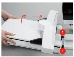
> To remove, lift the embroidery module on the left and carefully pull to the left.
