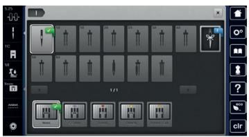
If the selected needle is suitable in combination with the selected presser foot, sewing can be started.
