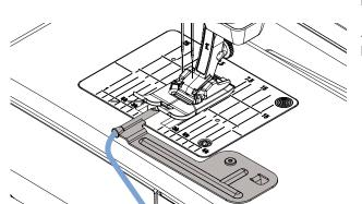
Sew delicate and decorative pin tucks easily with the cording attachment. The tube on the attachment provides ample room for a cord to be inserted for sewing raised pin tucks.
