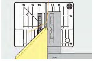
Correct this by placing one or more plates close to the edge of the fabric.
