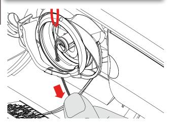
The bobbin can be filled with different thread, ribbons or cords, e.g. perle yarn and metallic threads, narrow satin ribbon, elastic threads and wool threads for free-motion stitching to add texture. This method is similar to "normal" free-motion sewing, but is done on the wrong side of the fabric
