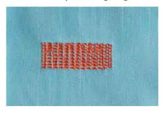
If the darning becomes distorted Correct with the Balance function see **Preparation**
