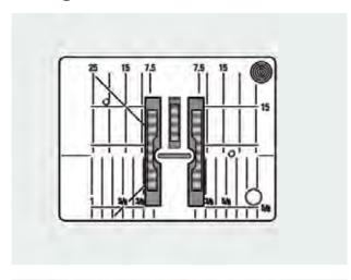
Due to the width of the stitch plate hole the outer feed-dog rows are relatively far apart.
