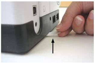
Please remove the protective sticker of the battery before taking the sewing computer in use.
