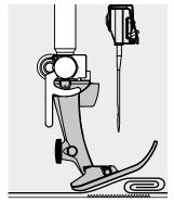
The feed-dog works accurately if the presser foot is level.
