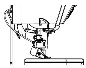
attach the BSR Presser Foot to the sewing computer and plug the cable in the outlet provided
