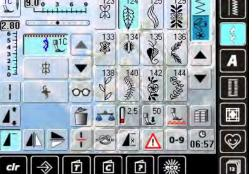
to add a pattern at the beginning of a combination, the cursor must be positioned above the first pattern
