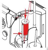
Any of the two spool pins (see arrow markings) can be used. However, it is best to use the rear pin due to its more favourable unwinding angle. Refrain from using the pin of the winder.
