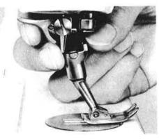
Release fixing lever and remove presser foot.
