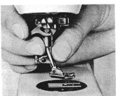
Fit required presser foot and press fixing lever downwards.
