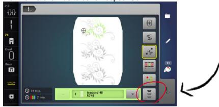
3) The embroidery hoop is moved near the last stitch. Via the multifunction knobs the horizontal and the vertical position of the needle in the embroidery hoop can be adjusted so that it is positioned exactly over a reference point.
