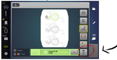
3) The embroidery hoop is moved near the last stitch. Via the multifunction knobs the horizontal and the vertical position of the needle in the embroidery hoop can be adjusted so that it is positioned exactly over a reference point.
