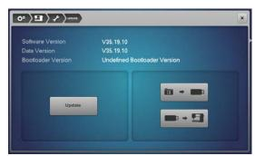
5.6. The Update procedure will be started and takes some minutes. Please do not switch off the machine or disconnect the USB-Memory Stick while the update is running.
