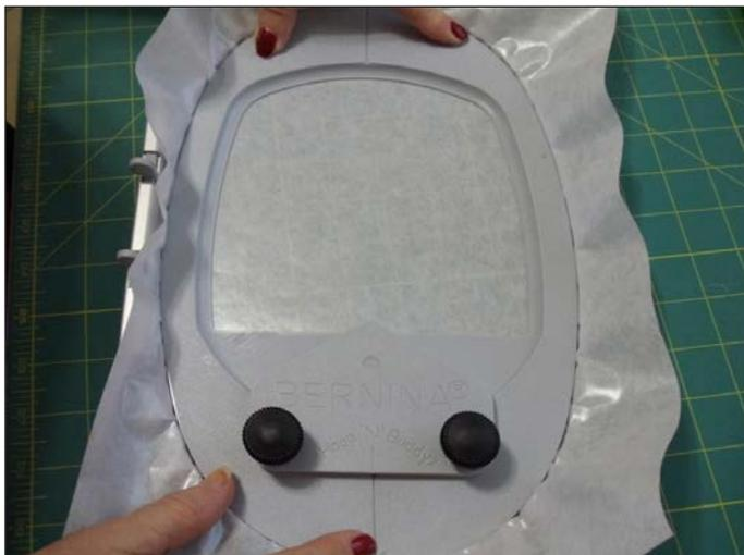
Make sure that the arrow on the hoop insert and the arrow on the outer hoop ring align. This indicates the Hoop 'N' Buddyz insert is correctly inserted.
