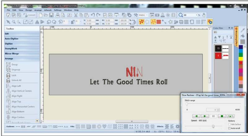
With lettering, stitching should begin at the bottom line of stitching in the center of the word and stitch out to each side.
