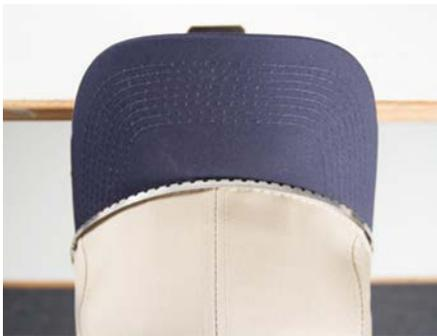
Take care to hoop the cap straight, even the slightest fraction off can make the design appear crooked. The strap on the cap frame should fall into the seam of the cap. If the strap has teeth they will be seated in that seam holding everything secure and straight.
