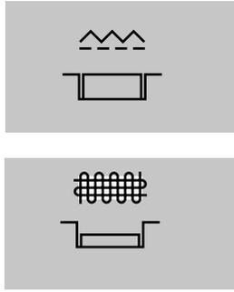
Button flush with housing = sewing position.
