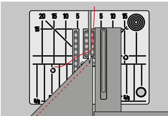
Correct this by placing one or more compensating plates as close as possible to the edge of the fabric.
