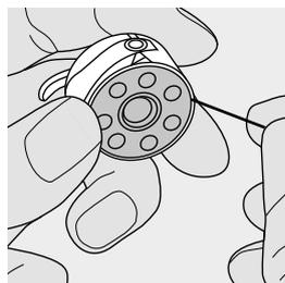
Insert the bobbin so that the thread runs clockwise.
