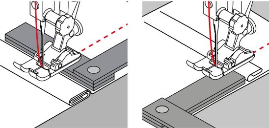
To solve this problem, place one, two or three compensating plates as required behind the needle under the presser foot to level it.
