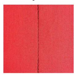
Due to a determined number of 6 stitches sewn forwards and 6 stitches sewn in reverse, the securing is regular.
