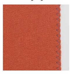
Zigzag No. 2 is suitable for all fabrics. It can also be used for elastic seams as well as for decorative work. Use darning thread for fine materials. When sewing satin stitch it is recommended to select a dense, short the zig zag with a stitch length of 0.3 – 0.7 mm. The satin stitch can be used for appliqué and for embroidering.
