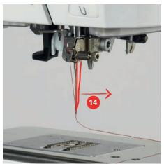
Pull the thread beneath the presser foot from back to front over the thread cutter (15) and cut.
