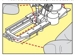
> Pull the cord on the left side under the Buttonhole Foot with Slide to the front.
