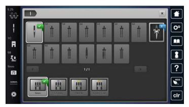
When the selected needle matches the selected presser foot, sewing can be started. If the selected needle does not match the selected presser foot, there will be an error message when starting the machine and the machine will not sew.
