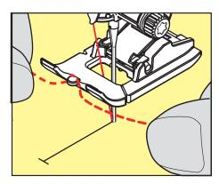
> Pull both cords ends under the Buttonhole Foot to the back and place each a cord into a groove of the sole.
