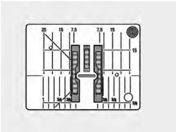
Due to the width of the stitch plate hole the outer feed-dog rows are relatively far apart.
