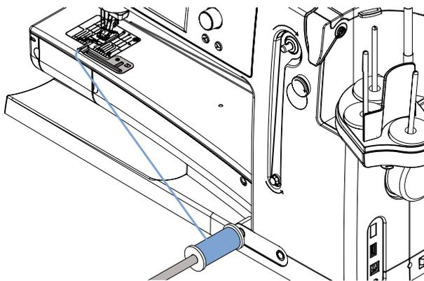
To help with even flow of cording, put the cord spool on the Free Hand System, so it doesn't fall on the floor or tangle while you're sewing.
