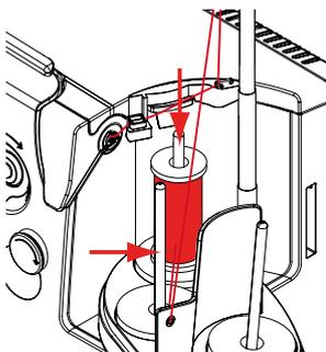
Any of the two spool pins (see arrow markings) can be used. However, it is best to use the rear pin due to its more favourable unwinding angle. Refrain from using the pin of the winder.
