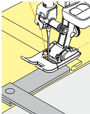
To level the presser foot as required, place one, two or three height-compensating plates behind the needle under the presser foot.
