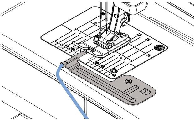
Sew delicate and decorative pin tucks easily with the cording attachment. The tube on the attachment provides ample room for a cord to be inserted for sewing raised pin tucks.
