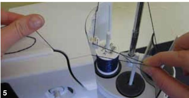
► place thread spool on spool pin and guide thread through thread guide. Then run thread via middle eyelet of telescopic rod. Continue threading the sewing computer as normal
