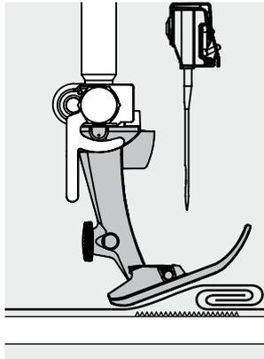
The feed-dog works accurately if the presser foot is level.
