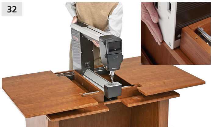
32 Position the machine onto the machine base support. The back of the machine should be positioned so that it is flush with the back of the top base frame.
