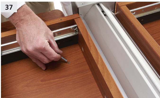
37 Insert the base mounting bracket bolts (J) through the top base frame surface (on both the left and right sides) and through the base mounting bracket. Secure by positioning the washer and nut.
