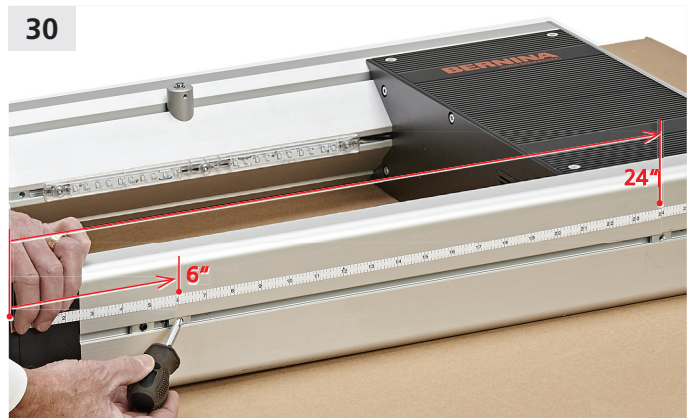
30 Position the Q 20 on its side and slide the internal machine mounting bolt brackets from the front edge 6" (15.24 cm) for the front bracket and to 24" (60.96 cm) for the back bracket.
