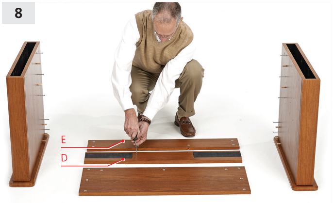
Screw camlock pins into back support (E) camlock holes, flush to the surface of (D) base support, using screwdriver (P).
