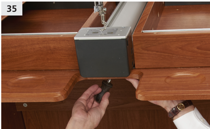
35 The front base mounting bracket will need to be secured from underneath the table.
