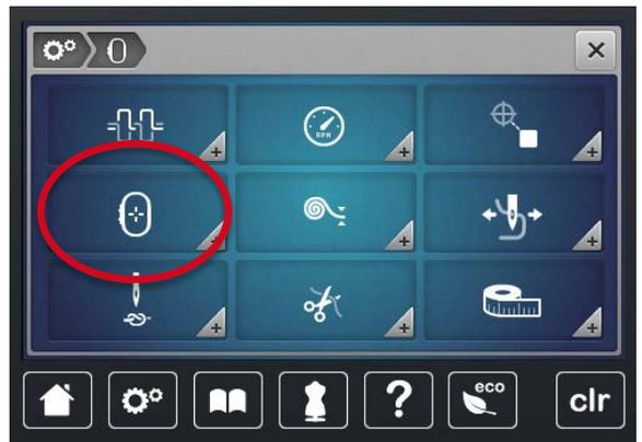
When prompted, attach hoop with the grid template inserted. The machine will then move to the centre position. Check the needle is sitting over the centre hole of the grid template. If the needle isn't centred, use the onscreen arrows to adjust. Once adjustments are complete, press the green tick.
