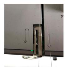
Also it is a good idea to leave one of the threads out of the last thread guide on top of the needle.
