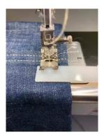
Stitch slowly, moving the tool towards you with every stitch. As soon as the back of the foot is off the seam, remove the tool.
