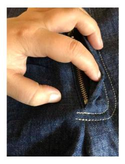
After that fly front stitching is complete, you can use the bar tack program to secure the fly guard. The bar tack program is a small satin stitch that has a pre-determined length. The stitch can be found in your utility stitch menu (check your manual for exact location on your machine).
