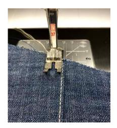
One of the major advantages in using foot #37 is the markings on the side. The markings on the side of the foot are a ¼ inch apart and can be used as guides when turning corners.
