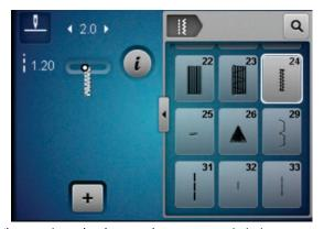
When using the bar tack program, it is important to trust the machine. Keep your foot on the foot control as it will stop itself when finished. Do not try and predict where it may end as the machine will do this for you.
