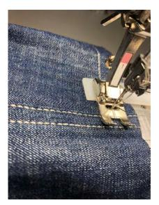
Stitch over your seam, keeping the tool at the back. As you come off the seam, move the tool to the front of the foot to level it out.
