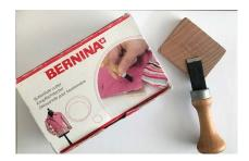
Place the buttonhole over the wooden block, take the blade and carefully press into the buttonhole split.
