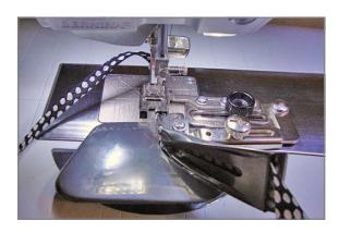
Stitch them in place using Edgestitch Foot #10/10C/10D and a needle position 2-3 steps to one side.
