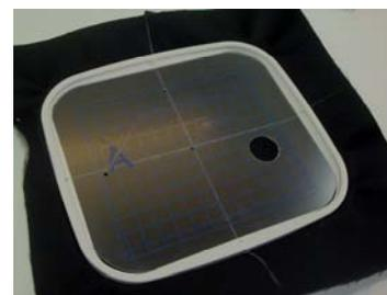
Use the plastic template that fits into the hoop to check the alignment.
