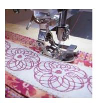
Using Edgestitch Foot #10D, sew the layered border to the front of the wall hanging along the edge of the background fabric. Guide the edge of the fabric along the center blade and adjust the needle position to stitch on the fabric.
