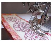
right toe of the foot to use as a guide. Sew around all four edges of the felt rectangle.
