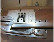
Attachment secures to the bed of machine and can be attached to the right or left of the needle as needed. Directional stitches and letters will be mirror imaged when stitched from each side
