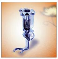
The vertical spring action of this presser foot works with the exclusive BERNINA hopper mechanism of the machine to hold the fabric in place as the needle moves in and out of the fabric. Like other BERNINA Freemotion presser
