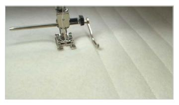
To eliminate marking, use the Quilting/Seam Guide on the back of the presser foot when channel quilting.
