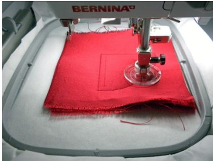
When the screen says Cut 2, turn the wheel on the CutWork Tool to Position 2 and resume cutting.
